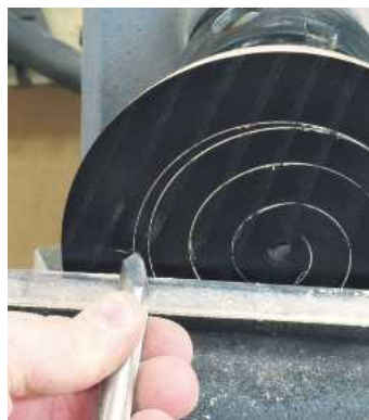
▲ Pic.8 One of the major problems when starting the hollowing process is overcoming the centrifugal forces involved. If you are not assertive enough with the tool, it will spiral towards the edge, as you can see here
